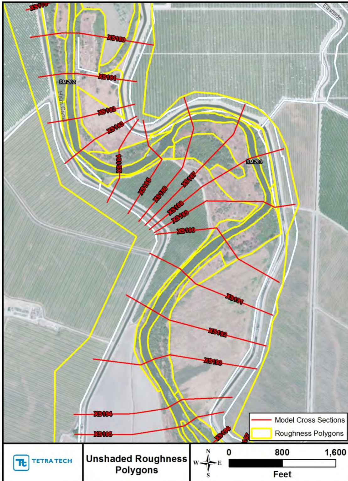
Figure 2.1. Aerial photograph of a portion of the project reach in the vicinity of RM 203.5, showing the un-shaded roughness polygons and hydraulic model cross sections.
