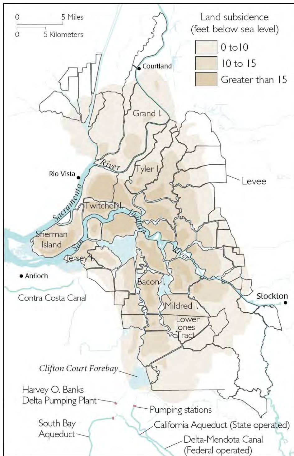
Figure A-4. Shaded contours of subsidence in the Sacramento-San Joaquin Delta and the Delta pumping plant (from Ingebritsen et al., 2000).
