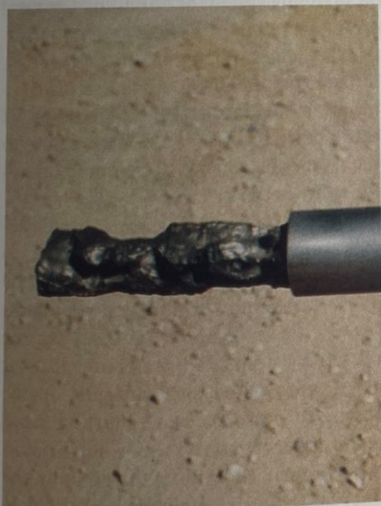
Figure 19.13. Destruction of this pump shaft has been caused by the creation of galvanic cells between the steel shaft and the bronze impeller. (Bergerson-Caswell Inc.)
