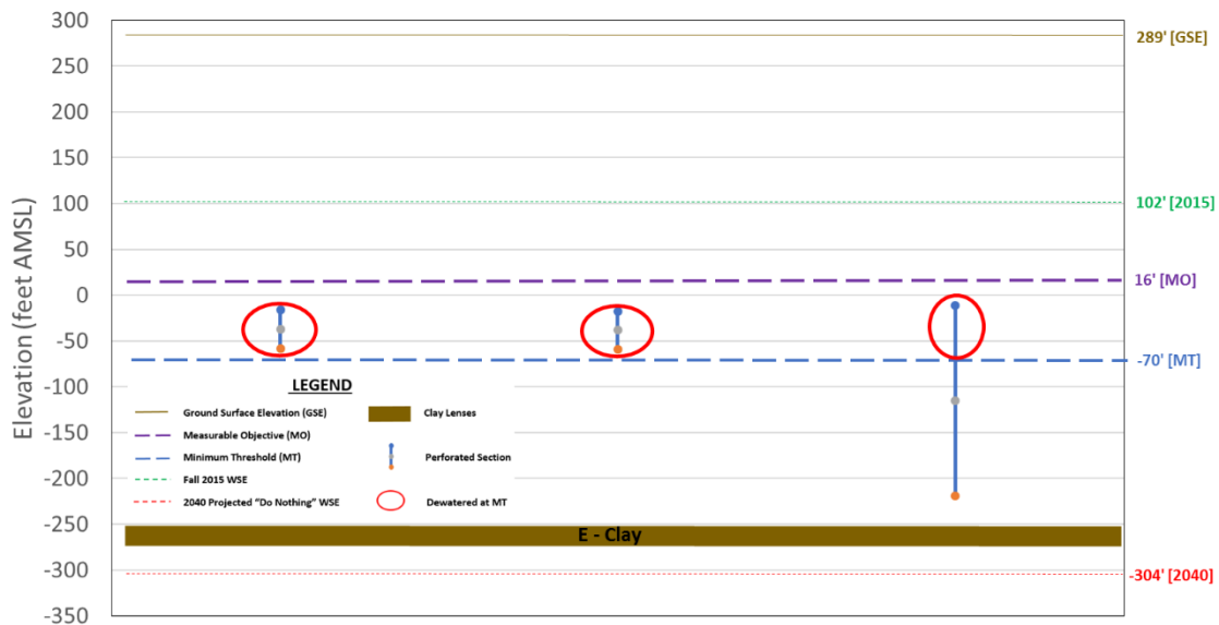
Figure 5-10i. Minimum Threshold and Measurable Objective Setting for DMW 12b
