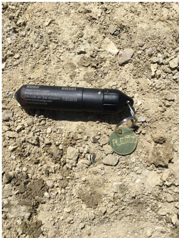
Figure 1. Typical HOBOT U20L data logger
