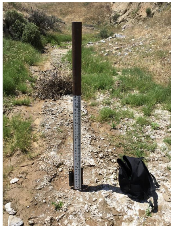
Figure 2. Typical staff gage. This one is located in Tecuya Creek
