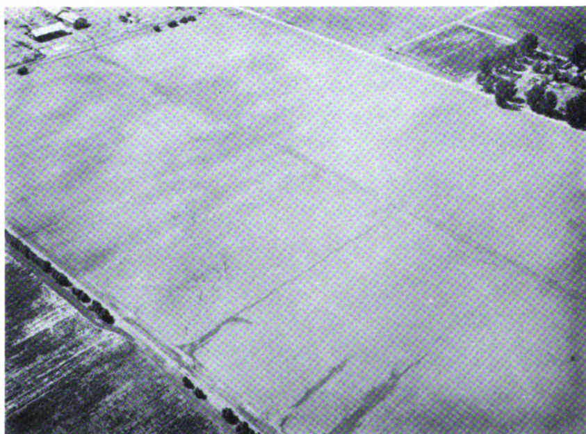
Photo No. 10—Cracking pattern in a plowed field about three miles southwest of Arvin. Swirl effect probably due to differential settlement of the sediments.
