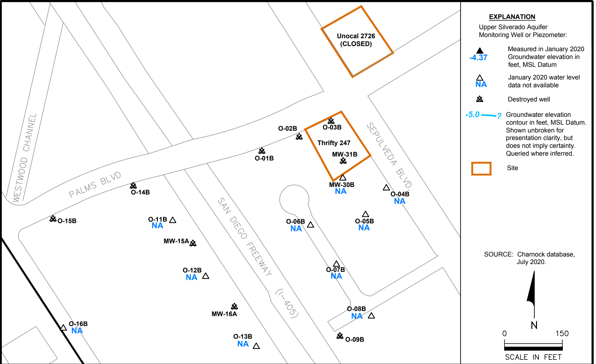
Potentiometric Surface Map - Upper Silverado Aquifer, January 2020 Palms and Sepulveda Intersection Detail Charnock Sub-Basin; Los Angeles, California
