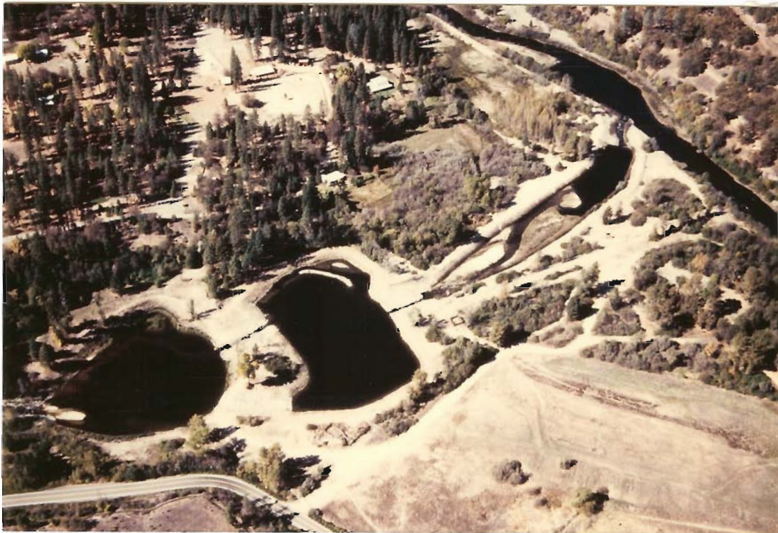
Sediment pools at the mouth of Grass Valley Creek stop the sediment from reaching the Trinity River.
