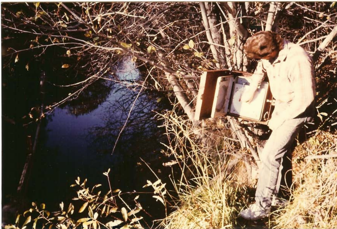
Thermographs were installed to record surface water temperatures during 1989 and 1990.
