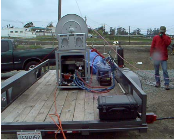
Figure 4: Electrical and Pneumatics components inside housing are controlled by the Dye Injection Control Unit (Figure 4). The housing contains injection pump, injection pressure regulator, pneumatically controlled valve switching solenoid, fuse box, electrical circuits and primary and secondary valve control units.
