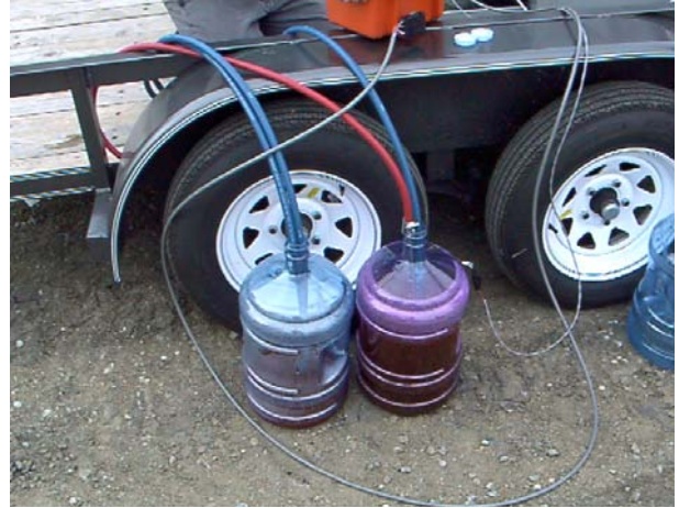
Figure 5: Bottle to right contains primary RR reservoir. When the large oval red button is depressed on the Dye Injection Control Unit (Figure 4), the RR solution is fed from the red tube, then to the injection pump, and finally through the injection nozzle and into the well. When the injection pump is idling, the RR solution circulates through the blue tube and red tube in the primary RR reservoir bottle. The secondary RR bottle receives excess RR that is not used during an injection pulse.
