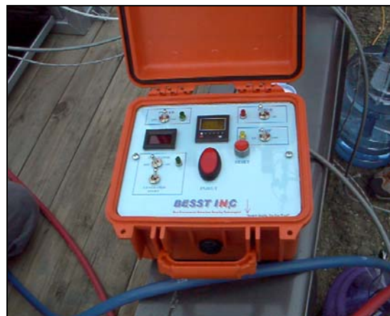
Figure 3: Injection Timer Control Unit used for pulsing tracer into well.
