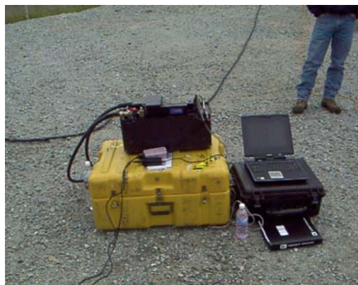
Figure 7: Laptop connected to 10-AU
