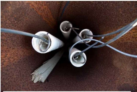
Inside a groundwater monitoring well. Kelly M. Grow / California Department of Water Resources
