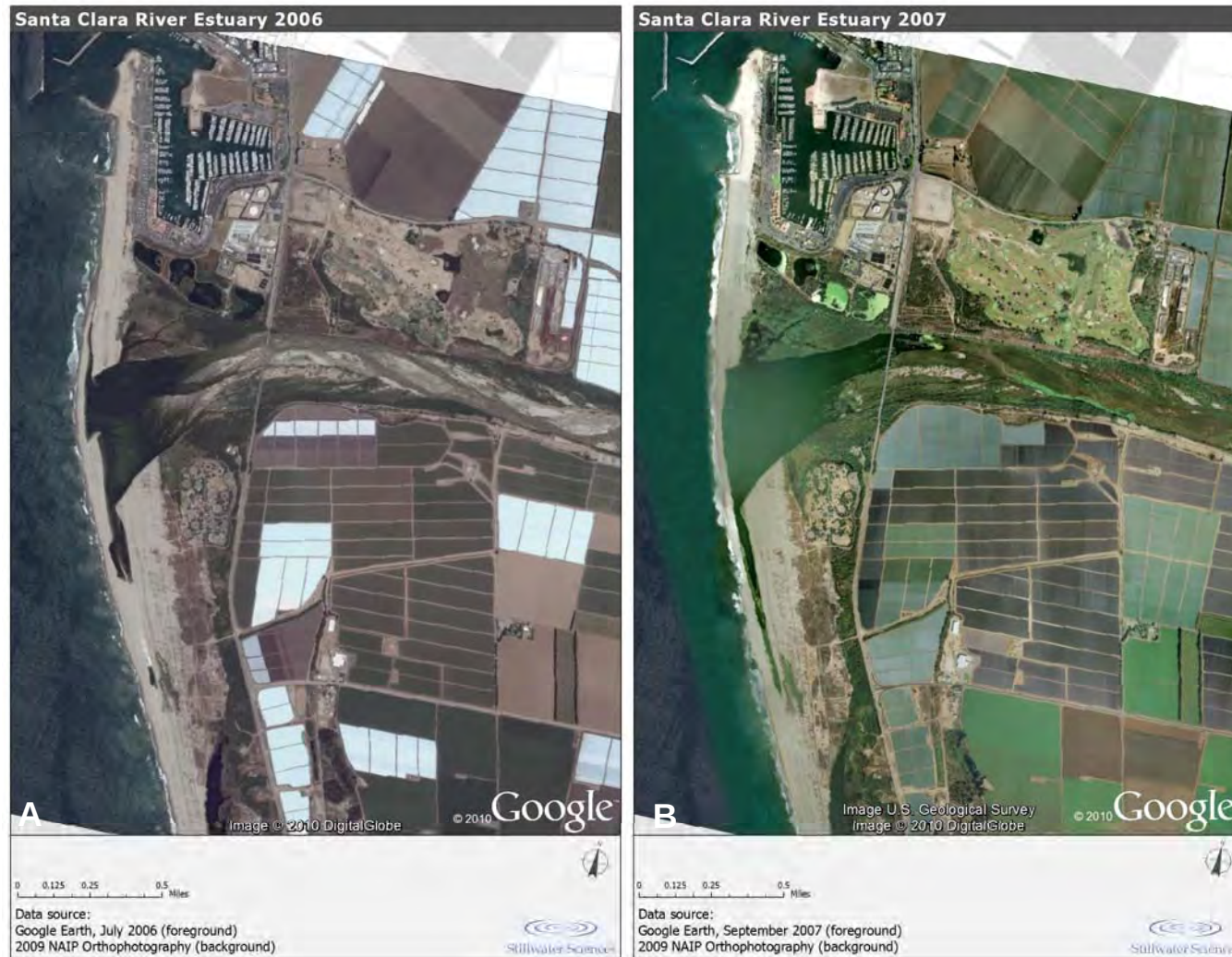
Figure 3-14. SCRE main channel, lagoon, and adjacent floodplain extent in the Present-day period following the 2005 flood events (July 2006 [A] and September 2007 [B]).
