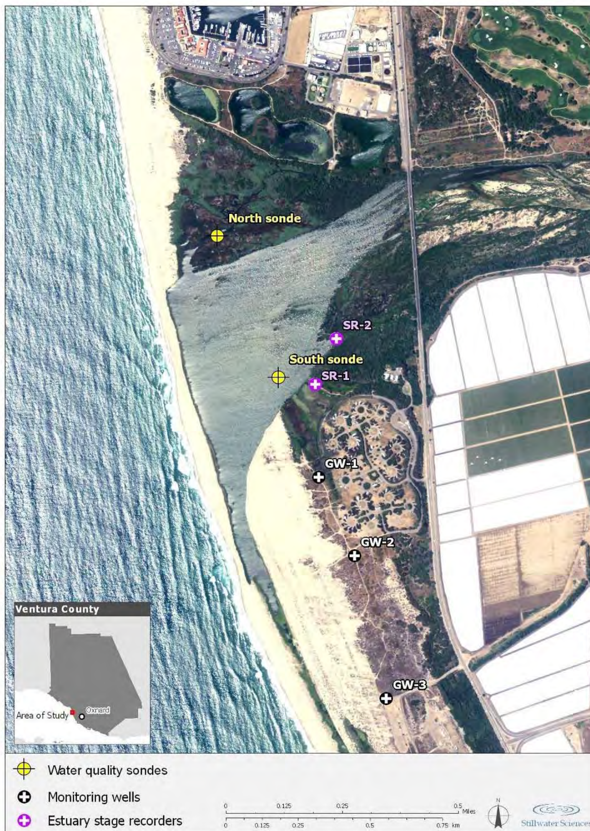
Figure 4-14. Location of SCRE stage recorders and groundwater monitoring wells.
