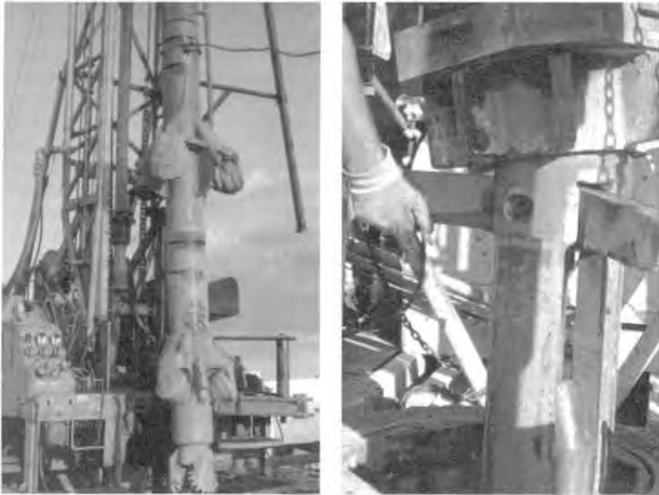
Figure 10.15. On the left, a three-tiered 48-in (1,220-mm) reamer bit has just been removed from the borehole. ( Snider Drilling Ltd. ) For soft sediments, underreamers (right) are constructed of blades that extend outward from the bit.
