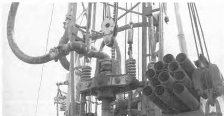
Figure 10.21. The upper end of the kelly connects to a swivel suspended from a traveling block in the mast. (E. H. Renner & Sons, Inc.)
