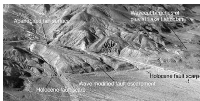
Figure 31. Older alluvial fan surface truncated by wave-modified fault scarp which records longer-term Quaternary uplift, and lesser scarps in younger washes which reflect most recent normal fault activity at Penrod Canyon. Perspective of photo is shown in Figure 29.
