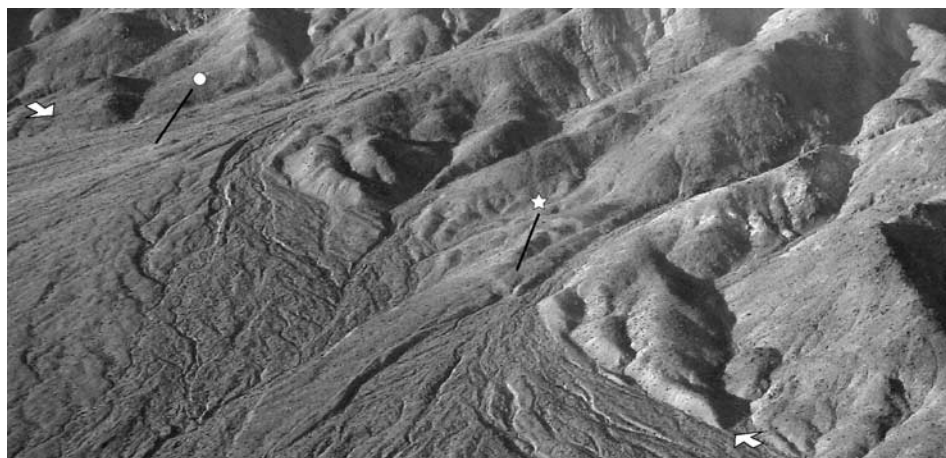
Figure 28. Oblique air photo of Indian Head fault trace (between arrows) along west flank of Indian Head Peak. Perspective of photo is annotated in Figure 24. Older elements of active fan preserve fault scarps (circle and star). Channel margin is dextrally offset \sim 6 m along fault trace (star).
