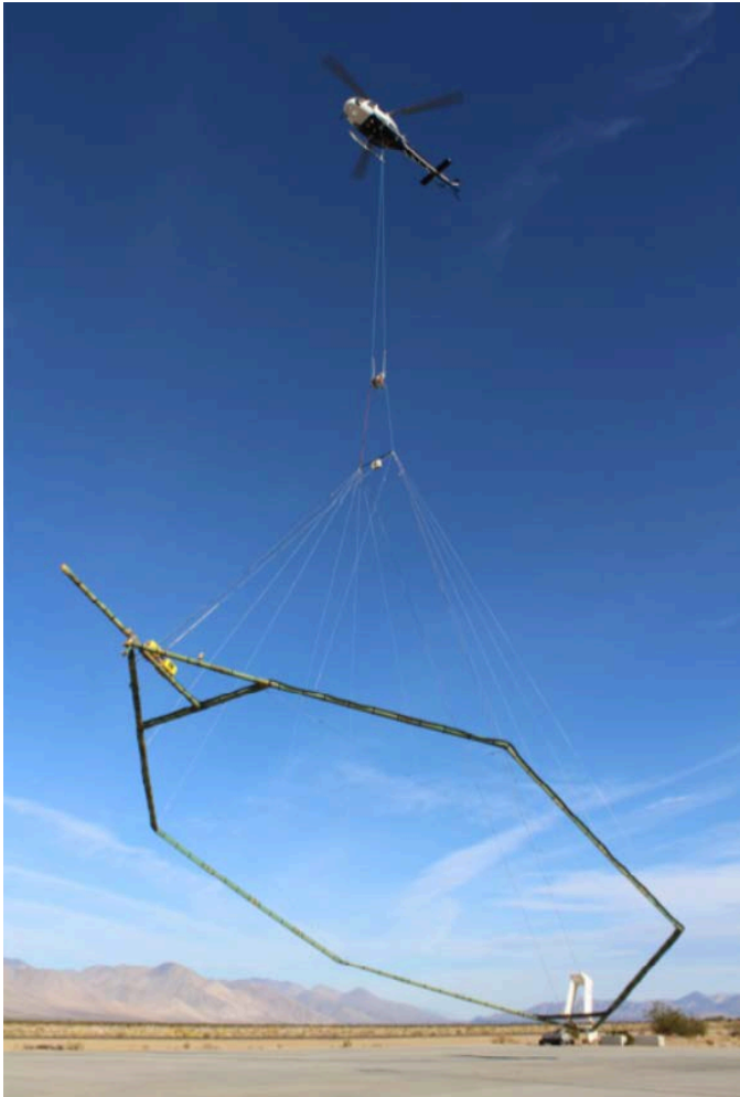
Figure 3-8. SkyTEM system during takeoff at Inyokern Airport.
