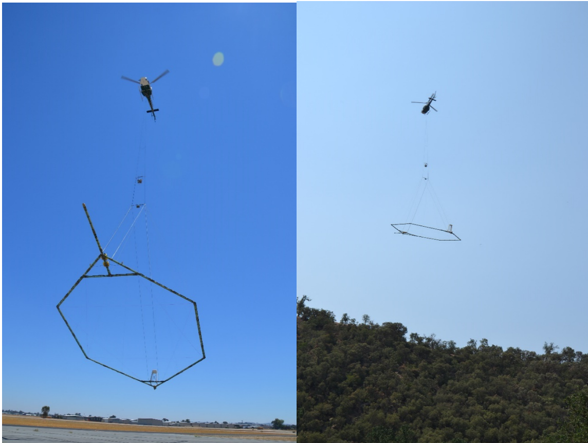
Figure 3-6 Photos of the AEM flights in the Salinas Valley Area. The top photo shows the AEM system resting at Paso Robles airport. The bottom left shows the system during take-off and the bottom right shows the helicopter towing the array during the survey.
